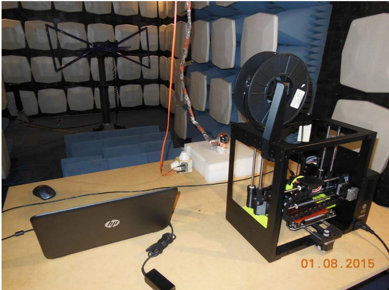
**Radiated immunity test setup – 80-1,000 MHz**
