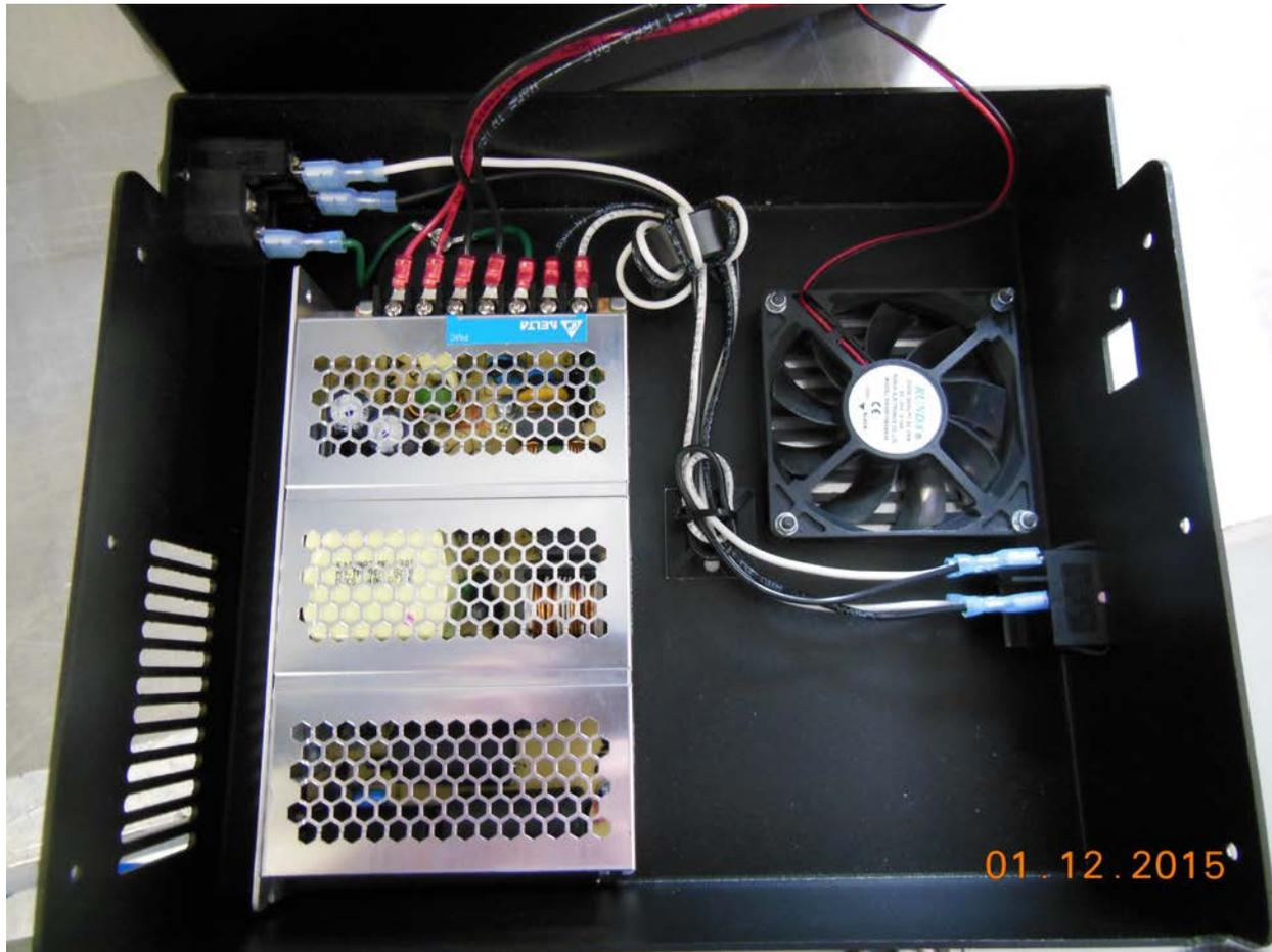
A ferrite was also added to Line and Neutral of the incoming AC power wiring as shown above.
