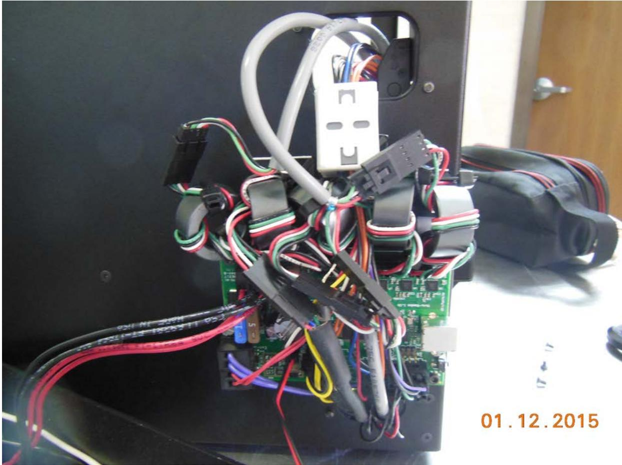
Ferrites were added to all the wiring as shown in the above picture.
