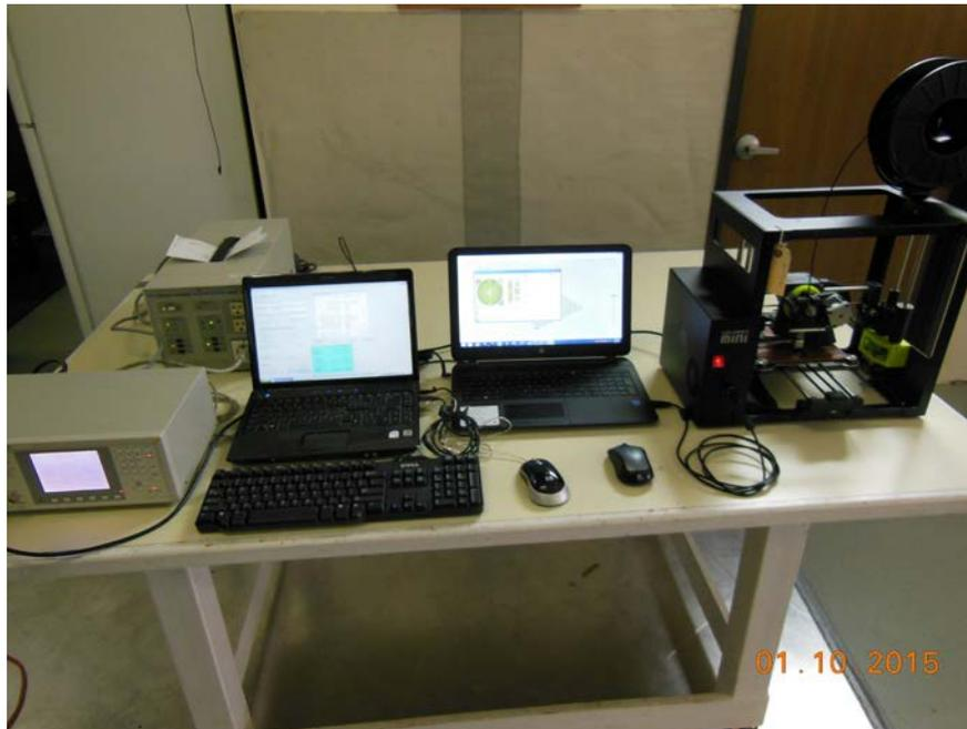
Test setup for AC power line harmonics
