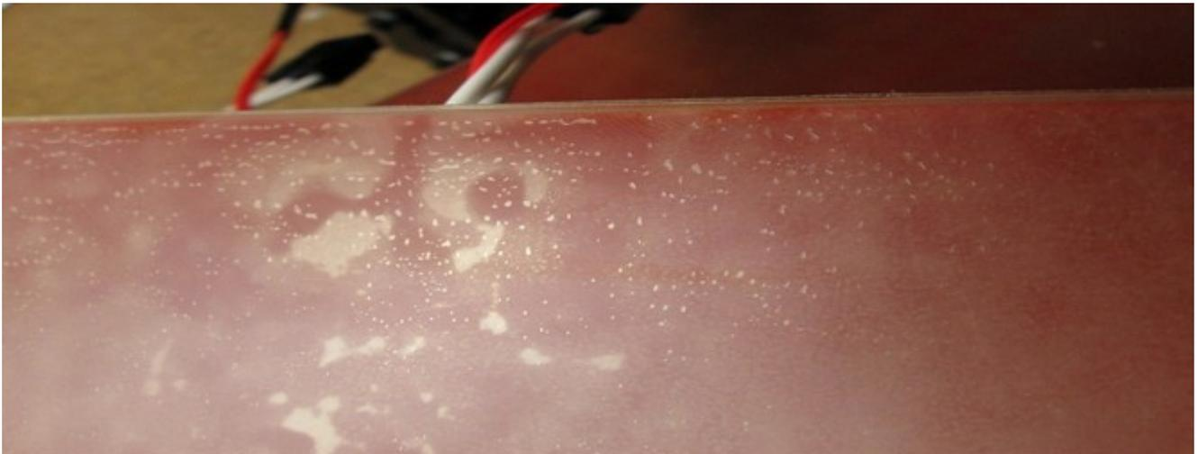
**Example of a passable amount of silvering. Note that the silvering is within 2" of the edge and that none of the bubbles are joining together.**
