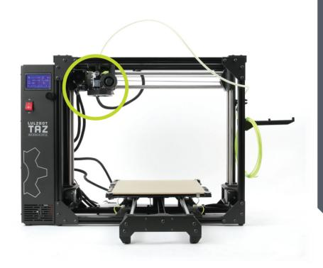
**6.4** Once the hot end reaches its wiping temperature, the tool head will move to the wiper pad (A), cleaning the nozzle of residual filament. After the nozzle has been cleaned, your LulzBot TAZ Workhorse will heat to probing temperature and conduct an automated self-leveling sequence by touching each bed corner (B). When the leveling process is complete, the printing process will commence.
