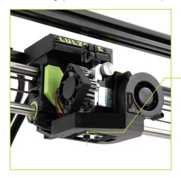
Very hot! Do not touch! **5.2** Once the hot end reaches the target filament removal temperature, the filament will automatically begin to retract. Once the filament stops moving, pull it out of the idler.
