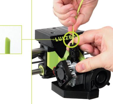
**5.7** With the PLA in place, press the LCD Control Knob to begin the purging process. Let the filament advance until it extrudes smoothly as shown. If the filament stops advancing and filament is not extruding from the nozzle, select **Purge more**, otherwise select **End filament change**.
