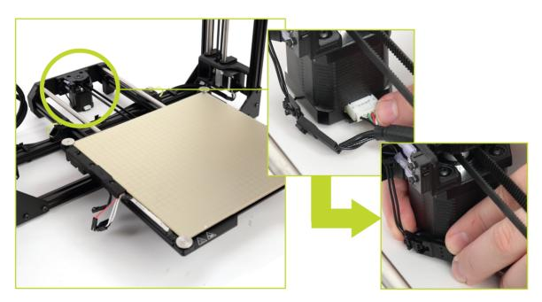
**3.6** Connect the three sets of wire connectors from the bed harness coming from the back of the control box to the left side of the bed as shown below. Start with the small two pin connection (A), then the small three pin connection (B), then the large heater connection (C).
