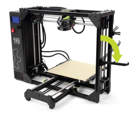
**5.4** Attach the filament guide tube to the feed tube holder, making sure that the guide tube and filament are behind the feed tube holder as shown. Feed the PLA filament up into and through the filament guide tube. Continue pushing filament through the guide tube until an easily grasped length is protruding from the other side.
