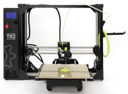
**6.6** Once finished cooling to the proper removal temperature, the tool head will move to the top right and the print bed will move forward. Once the print bed has stopped moving, remove your first calibration print by gently sliding the included blue-handled knife under each side, then under the center of the print until it separates from the bed.
