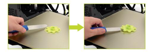
The blade of the blue-handled knife is sharp. Exercise caution when using it. The blade should be nearly parallel with the print bed and move parallel to the bed. Avoid prying prints up and away from the bed.
