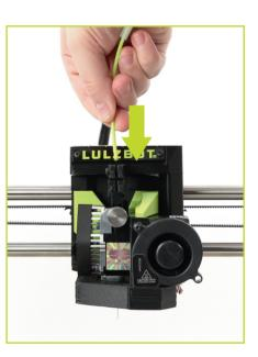
**5.5** Locate the filament guide tube holder and idler on the tool head where the loaded filament was removed during step 5.2. Filament feeds down this path and into the hot end for printing.
