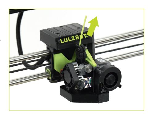
**5.3** Rotate the filament holder and filament guide tube holder into place. Once in position, place the included PLA filament on the filament holder.
