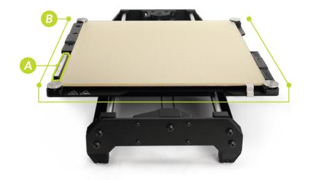
**6.5** After your LulzBot TAZ Workhorse is finished 3D printing, the tool head and print bed will automatically move into the cooling position with the tool head in the top left of the build area and the print bed fully back.
