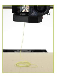
After removing filament, a small residual amount remains in the hot end that needs to be cleared out through the process detailed above. This purging process helps to remove any residual material left in the hot end.
