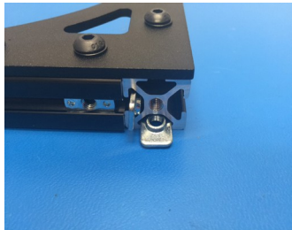
Two T nuts each added to the bottom and inside slots of the extrusion (left and Right)
