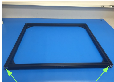
Position the back frame assembly, threaded extrusion toward you
