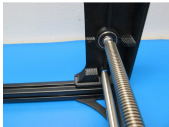
Install the X end left assembly to the Z top
