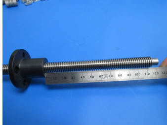
Install Z nut onto lead screw
