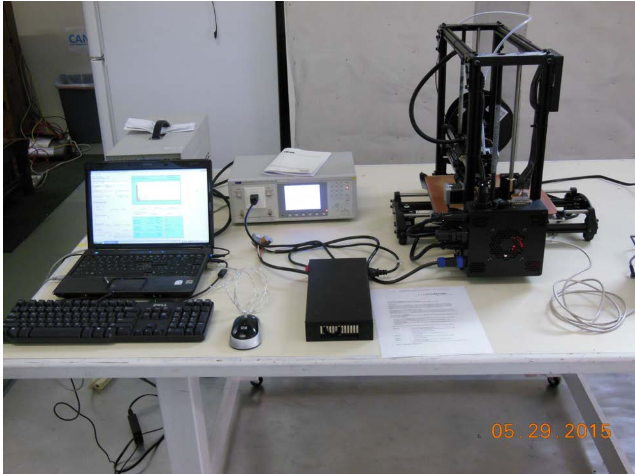
Test setup for AC power line harmonics
