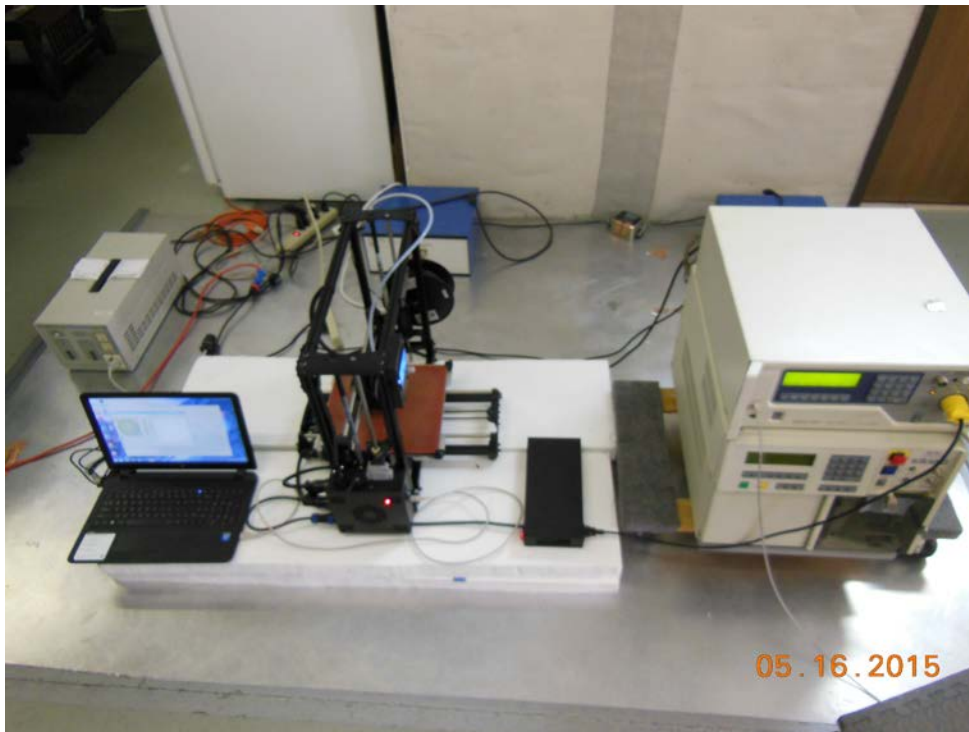
Test setup according to EN 61000-4-5, Surge
