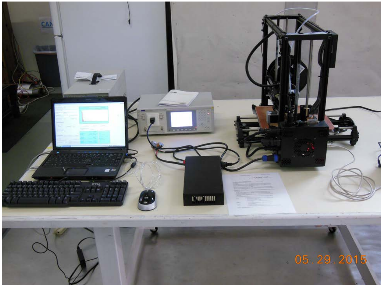
Test setup for Voltage fluctuations and flicker EN 61000-3-3
