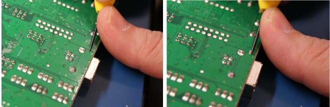
6.Place varistor or stencil over pad to check your progress and clear more solder mask as needed. We used hot air to perform this patch. For a soldering iron you will need to clear more mask.
