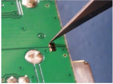
5.Use scraper tool (screw driver or sharp tool) to scrape the solder mask from the marked area. Take care not to damage the copper plane. It can help to rotate the board to clear the region. It is OK to leave the solder mask in the clearance between the two copper planes. This is also best under magnification.
