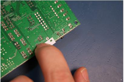
3. Fill stencil with sharpie. Hold stencil tight to prevent movement. Stencil shown (2mm x 1.2mm) is suitable for hot air. 3mm x 2mm stencil is better for use with solder iron.
