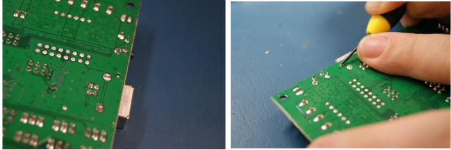
7.Add solder paste. (If using paste)8.Place varistor9.Use hot air (or iron) to solder.
