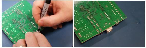
4.Use razor tool to cut a border around the stenciled mark. Be careful to only cut the solder mask. This step is best done under magnification.
