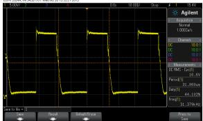
Note that the measured duty cycle is actually 44.182% but this is simply due to the non-ideal rise and fall times of the digital signal, and since the measurement is taken at  $V_{DD}/2$  the duty cycle is measured to be slightly higher. Also note that  $V_{RMS}$  = 16.6V whereas the calculated RMS value is 15.18V<sub>RMS</sub>.
