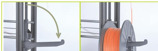
**A** Place the filament on the filament arm (front right hand side of the printer) with the filament feeding counter clockwise. Feed the end of the filament through the feed tube, through the PTFE sleeve and exiting near the extruder.
