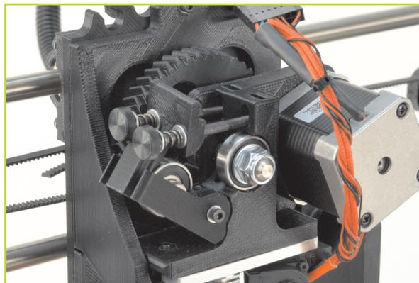
**C** Once the filament extrudes a small amount out of the nozzle, raise the idler and slide the two idler bolts and plate back into place. Tighten the two idler bolts. Tighten the two screws until the top of the thumbscrews are about 10-11mm away from the plastic clip.
