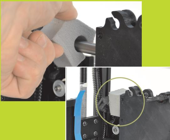
Locate and remove the gray foam block used to hold the X axis carriage in place during shipping.
