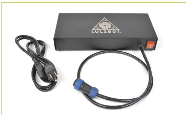
**10** Locate the blue 24VDC output cable plug from the power supply. Connect the blue power supply plug into the keyed power supply connector on the TAZ electronics enclosure. Once the plug is pushed in completely, turn the locking sleeve clockwise until it is tight against the electronics enclosure. Hand tighten only!
