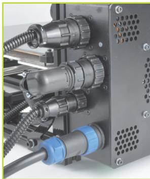
**12** Plug the AC power cable into the power supply. Then plug the other end into an AC power outlet.
