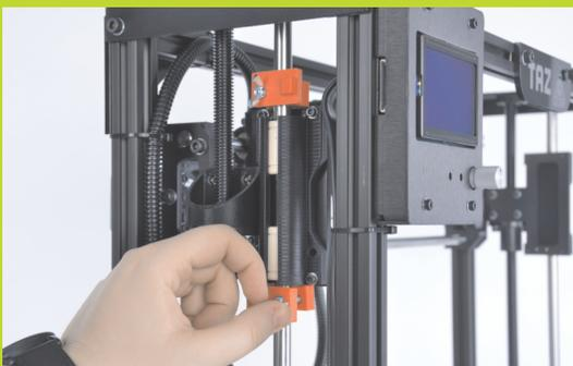
Remove red protective packing clips from Z and Y axis smooth rods.
