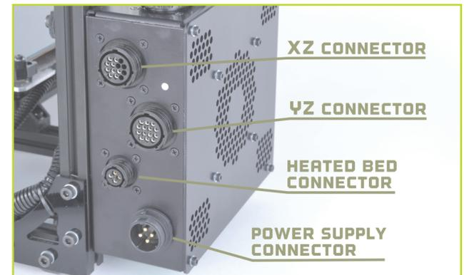
**8 cont.** The top most connector matches the large straight plug from the XZ cable. The next connector down matches the large angled plug from the YZ cable. The third connector matches the smallest plug, from the heated bed cable.
