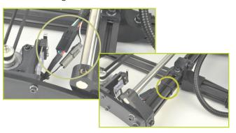
With the included 2.5mm hex driver, locate and remove the 3mm tool head screw in the top center of the X axis carriage. Next, take the tool head out of the Accessory Tray foam insert.
