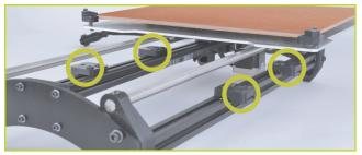
With the print surface facing up and the stepper motor end of the Y axis facing back, slide the Y axis assembly on to the Y axis mount brackets, aligning the holes on the brackets with the bolt holes on the Y axis assembly.
