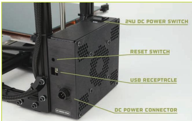
**11** Connect the DC locking plug into the DC connector on the TAZ electronics enclosure. The plug is keyed, which may require rotating the plug until the keys line up and the plug can be pushed in. Once the plug is pushed in, turn the locking sleeve clockwise until it is tight against the electronics enclosure.
