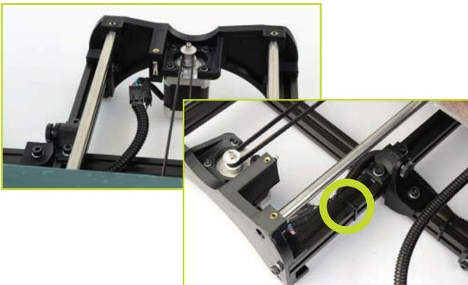
**6** Locate the two connectors to the left of the print bed. Connect the matching female and male large 2-pin heat bed connectors and the small 2-pin connectors.
