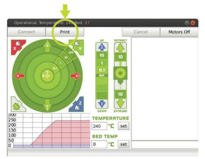
**11B** Your LulzBot Mini will first move its tool head to the top left corner and allow the hot end to cool down prior to starting its cleaning process. Depending on ambient air temperature, this can take 2-5 minutes.
