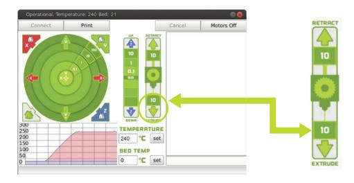
**10B** If you do not see filament coming through the nozzle and the drive gear stops moving, click the **Extrude 10** button once more and wait. Repeat as needed until you see consistent and repeatable extrusion.
