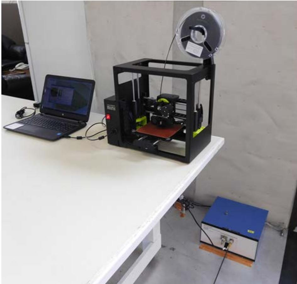
**Conducted emissions test setup**
