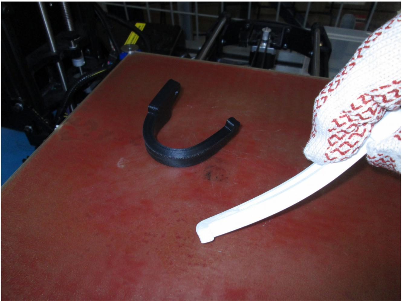
APLA (white) after being removed from a 135C oven exhibits some deformability, but impressively little. For reference the black ABS test piece was very easily bent into a u shape at the same temperature. Pretty cool.
