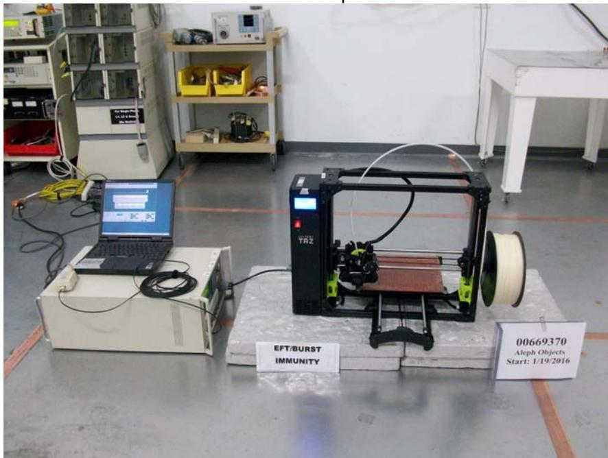
Test setup – AC Power
