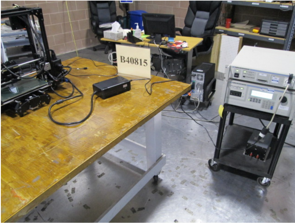
Figure I1. AC Power Line Flicker Test Setup.
