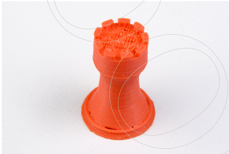
Figure 2.15: An example of insufficient top layers.
