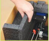
**A** While keeping printer in the box, pick up by the black aluminum frame and rotate the printer and foam 90 degrees — setting it upright within the box. Make sure name plate at top is UP. Remove top foam.
