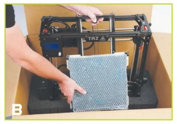
Carefully remove printer frame from box and set it on a sturdy, flat surface — you're ready for assembly!
