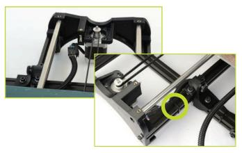
Locate the two connectors to the left of the print bed. Connect the matching female and male large 2-pin heat bed connectors and the small 2-pin connectors.
