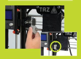
Locate and remove the gray foam block used to hold the X axis carriage in place during shipping.
