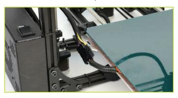
**T** Locate the two small black zip ties that are included in the documents bag. Wrap the two zip ties through the slot, located on the left rear of the aluminum bed plate, and around the print bed wires. Tighten the zip ties so the wire cannot move freely. Cut off the excess end of the zip ties with the needle-nose pliers included in the tool bag.
