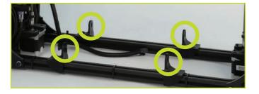
With the print surface facing up and the stepper motor end of the Y axis facing back, slide the Y axis assembly in between the Y axis mount brackets, aligning the holes on the brackets with the bolt holes on the Y axis assembly.
