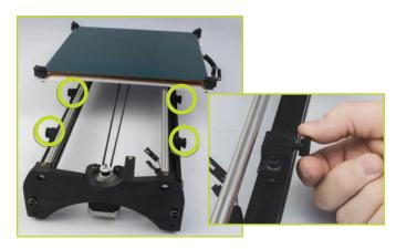
Locate the four Y axis mount brackets on the TAZ frame.
