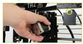
Connect the extruder assemblies' 4-pin connectors: match the orange/red wire connector pair for the hot end and the mixed color wired connector pair for the extruder motor. Connect the matching pairs together so they lock and click.
