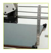
button. Turn the threaded rod on one side of the printer to raise or lower that side to match the measurement on the other side.
