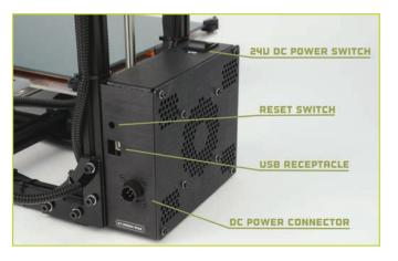
11 Connect the DC locking plug into the DC connector on the TAZ electronics enclosure. The plug is keyed, which may require rotating the plug until the keys line up and the plug can be pushed in. Once the plug is pushed in, turn the locking sleeve clockwise until it is tight against the electronics enclosure.
