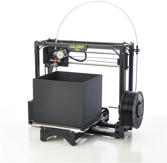
Figure 5.6: LulzBot TAZ 1.0 Max Build Volume.
