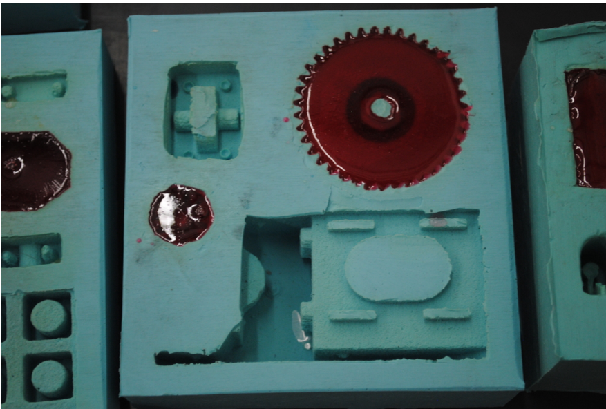
Figure 2.3: LulzBot Clonedel gears in the silicon mold.
